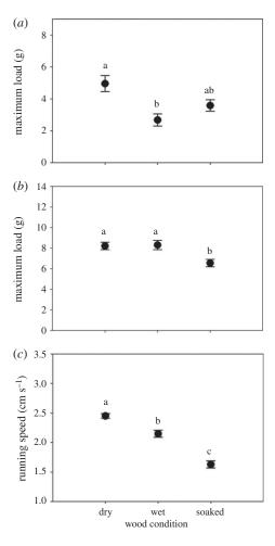
**Figure 4.** Static normal adhesion (a), static shear adhesion (b) and running speed (c) on dry, misted with water drops (i.e. wet) and water-soaked wood. Treatment groups denoted with the same letter are not significantly different.
