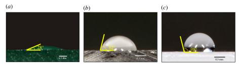
**Figure 2.** Example static water contact angle (SWCA) droplet images on hydrophilic glass (*a*), intermediately wetting polycarbonate (*b*) and hydrophobic polypropylene (*c*).
