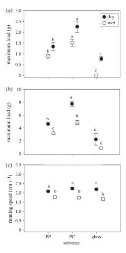
**Figure 3.** Static normal adhesion (a), static shear adhesion (b) and running speed (c) on three smooth, artificial substrates that vary in substrate wettability (static water contact angle ca 27°, 85° and 100° for glass, polycarbonate (PC) and polypropylene (PP), respectively). Treatment groups denoted with the same letter are not significantly different.
