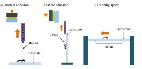
**Figure 1.** Schematic of the static normal adhesion (a), static shear adhesion (b) and running speed (c) experimental methods. Arrows indicate the direction of pull in (a,b), and direction of running in (c). Insets in (a,b) depict the contact interface where the fluid-covered tarsi (green = fluid, tarsi = grey) contact the substrate (blue). Arrows indicate loading direction.
