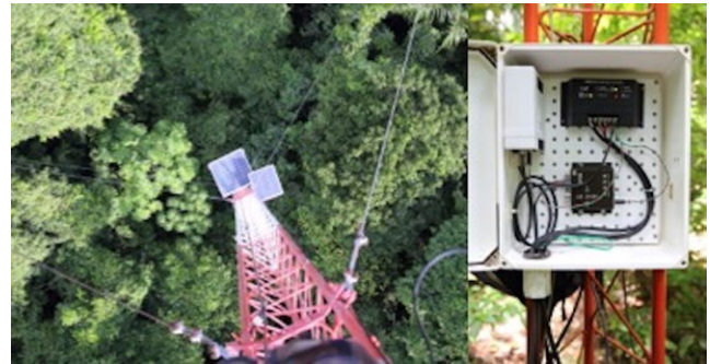
FIGURE 2 The solar panels (left) and electronic equipment (right) used to support individual cameras in the video network. The panels collectively provided up to 90 W of power to recharge a deep-cycle 12-V battery (not shown) during the day, while also powering the camera, GPS antenna, text overlay unit, and DVR. These latter components were then powered by the battery through the night
